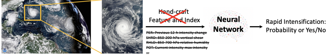
Figure 1: End-to-end Rapid Intensification Prediction. We propose to directly predict RI from raw climate data without intermediate heuristic hand-craft features.
